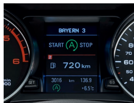
The start-stop status is shown in the Driver Information System display, which renders green during economical driving and red at other times
